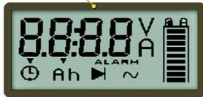
LCD DISPLAYING CHARGING DATA AND FAULTS, IF ANY
